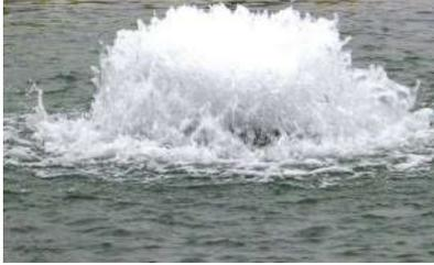
This is the aerator located behind Ketch Place that increases the oxygen content of the water in it's vicinity. Prior to the aerator there was a stagnant area of water in one corner of the beach behind Bartel Boulevard and Ketch Place.
